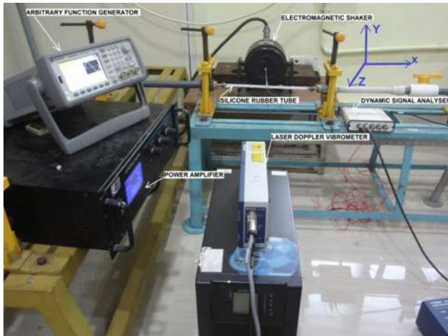
Fig. 2. Experimental setup used for the study of dynamic characteristics of the flexible tube.
